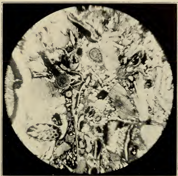
PLATE LXI.—Photomicrograph.—Dark-gray oolite, Union Limestone. x about 20. (Photo. by A. Berg and W. E. Rumsey).
